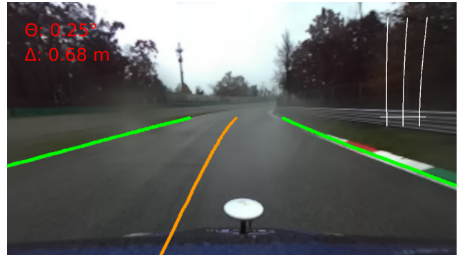
Fig. 1. Overview of the output of our system: lateral lines (green), centerline (orange) and relative pose heading and lateral displacement (red). On the right, reconstructed world representation of the scene.
