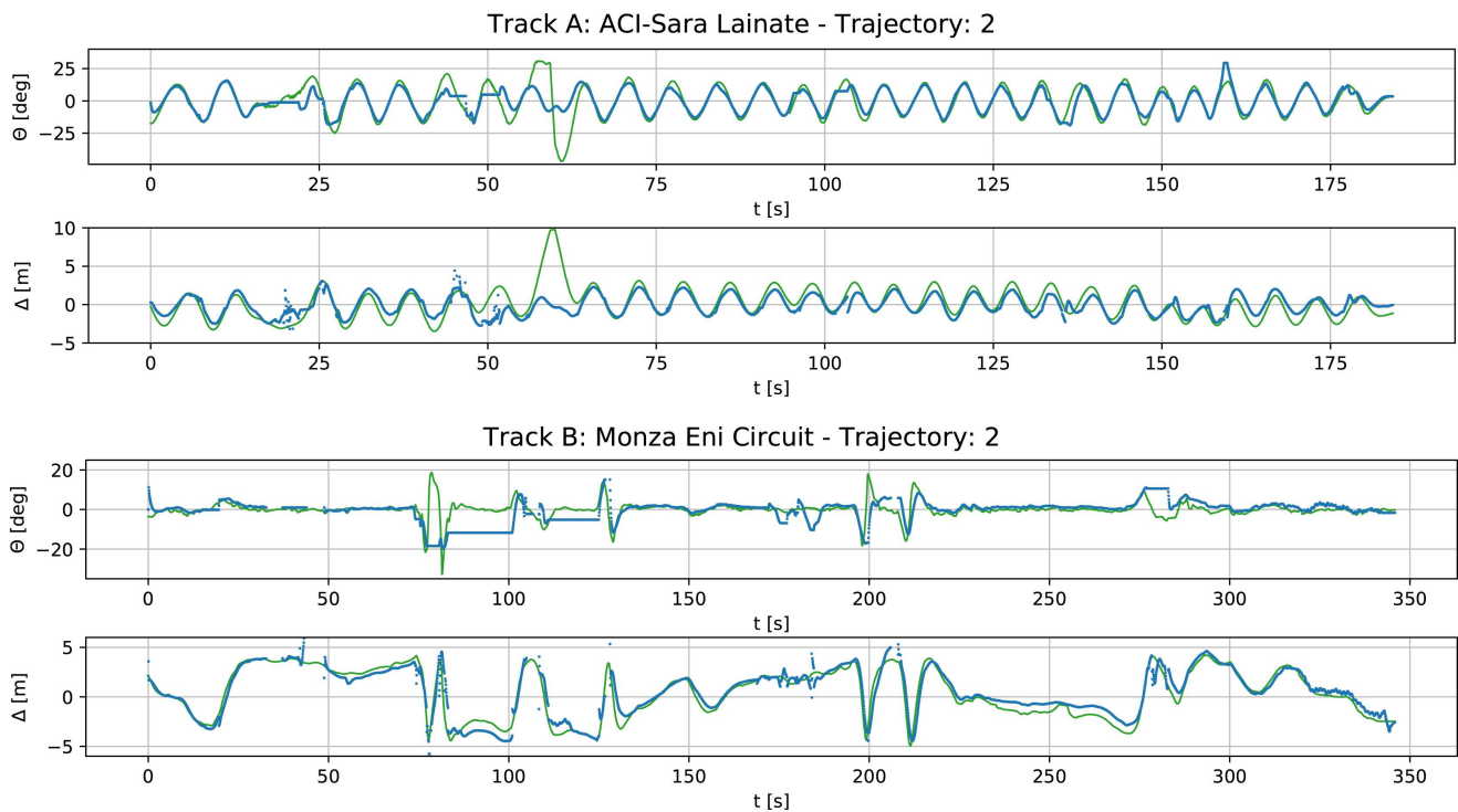
Fig. 8. Examples of the experimental results obtained in oscillating and racing driving styles, designed to stress the estimation of, respectively, heading (top) and lateral displacement (bottom). The graphs compare the estimates (in blue) with the respective ground truth (in green).
