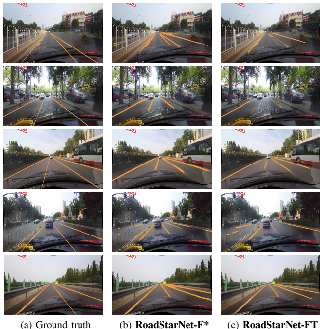
Fig. 3. Example of qualitative results: comparison of RoadStarNet single-class line detection output using different training functions on images from the CuLane dataset [10].
